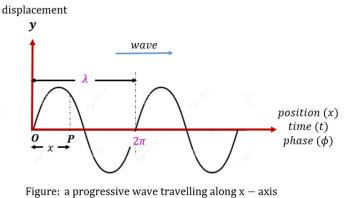
first vibrating particle, the equation of motion is written as:
