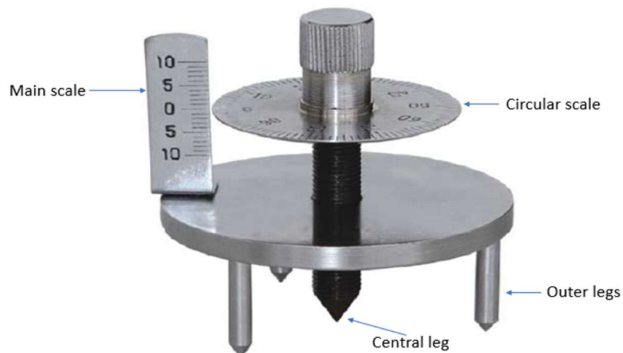
Figure: A Spherometer
