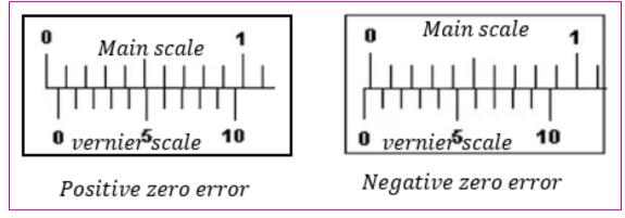
When two jaws of vernier callipers are brought in contact, the zero of vernier scale may or may not coincide with the zero of main scale. If the zero of main vernier scale exactly coincides with zero of vernier scale, then the calliper is said to have no zero error. But if the zeros do not coincide, then the calliper is said to have zero error.
