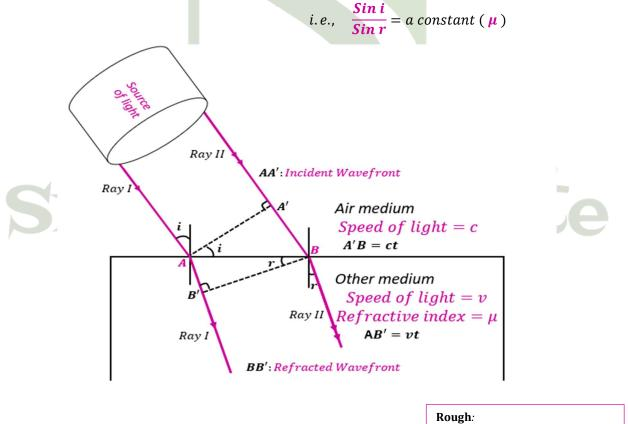
Width if incident wavefront = AA'Width if refracted wavefront = BB'
