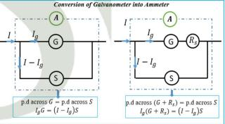
G =Resistance of Galvanometer coil, S = Shunt,  $I_g$  = Current across Galvanometer  $R_s$  =Series Resistance, The equivalent resistance of ammeter is  $\frac{1}{R_{eq}} = \frac{1}{5} + \frac{1}{6}$
